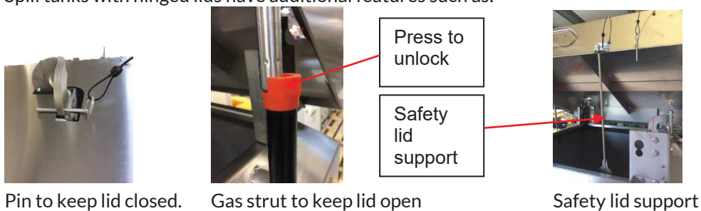
Fig 1.2c,d & e typical example of Spill tank features
