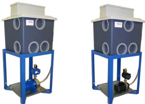
MonoMatic MM-FS-APT225: Single pump Fixed speed booster with controller "Presscomfort" or "PM2" and 225 litre break tank.
