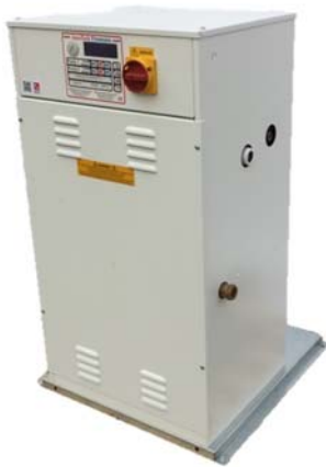
AquaPack AP3-DG (3.0Bar max cold fill) or AP6-DG (6.0Bar max cold fill) Twin Pump Pressurisation unit with (70°C continuous rated) Automatic Degassing feature built in.
