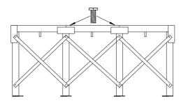
The upstands generally have a metal plate to support the base of the tank. Alternatively there may be a plywood base which should then be inserted into the top section before the tank is placed or
