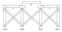
This then allows the centre section to be inserted into the middle. All of the remaining bolts can now be inserted and all of the feet should be bolted down.
