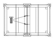
The upstands generally have a metal plate to support the base of the tank. Alternatively there may be a plywood base which should then be inserted into the top section before the tank is placed or assembled on top.
