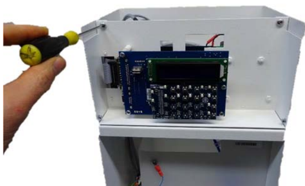
Fig 1.5a Control shelf retaining screws.
