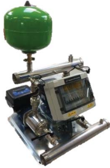
MicroMatic: HM2AV twin pump end suction Variable speed booster set with Flow Through Vessel & E-SPEED Motor Control
