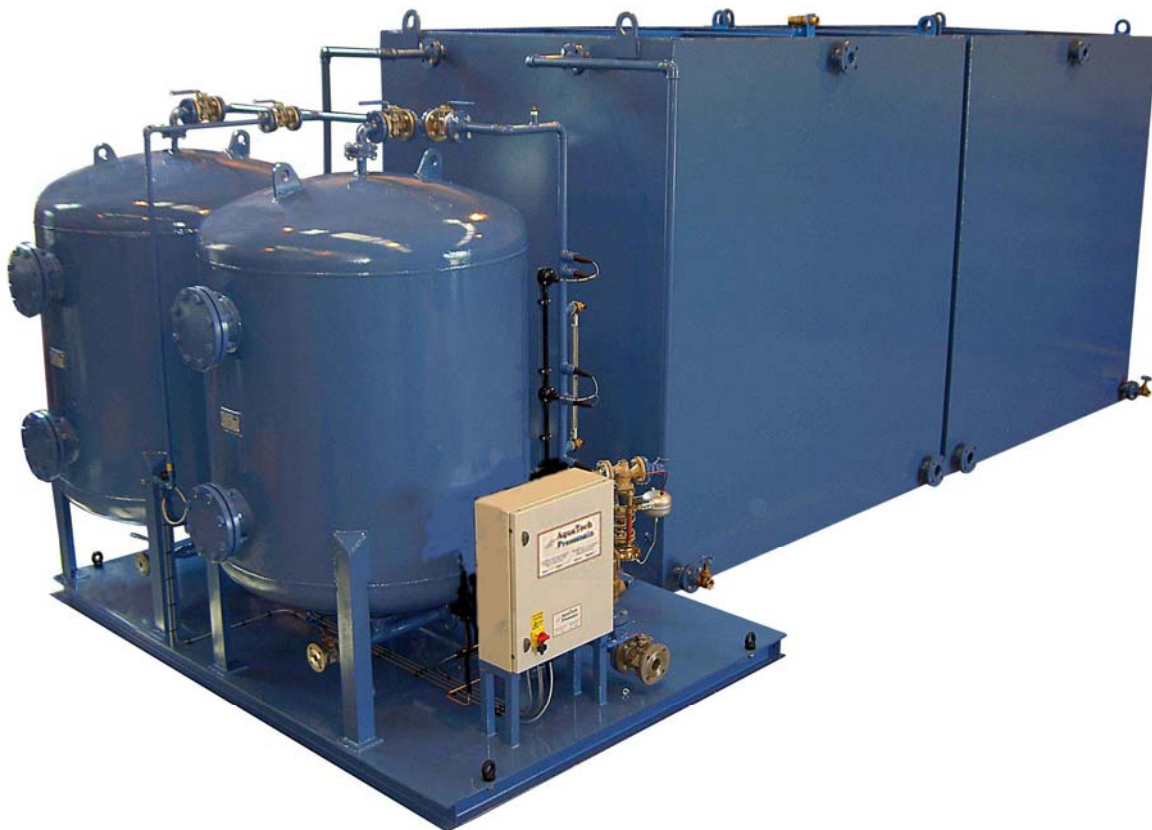
Fig 1: Example of a “SR2-E” High Temperature Hot Water heating system pressurisation unit, featuring duplicate Nitrogen control vessels and Spill valves etc, to ensure continuous operation in a critical application.
